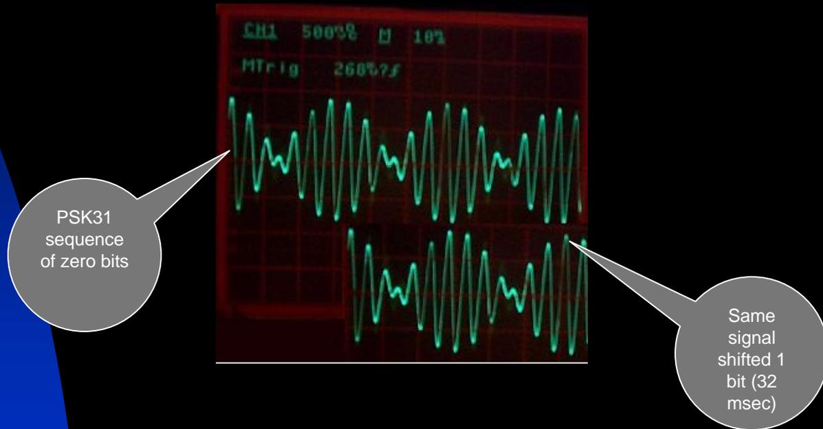
Notice that when we shift the signal one bit width (32 msec), and compare, the phase shift of 180 degrees is clear. This also gives us a clue for how PSK-31 is detected and converted back to the digital world.
