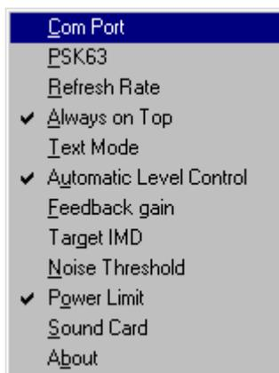
By clicking on Com Port, you will be able to set which com port PSKMETER uses to communicate with the hardware. There are a variety of options and configurations, as well as restrictions, you should be aware of when setting the com port:
