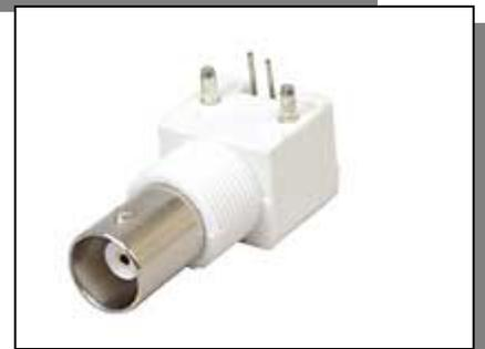
Insert the BNC connector J1 at location J1. There are two leads on this connector, and also two posts. Solder the two leads, but also apply some solder to the two posts. The posts have no electrical significance, but they add mechanical strength and integrity to the connector.
