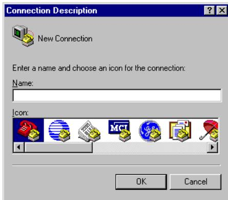
Open Hyperterm by clicking on Start, Programs, Accessories, Communications, Hyperterm. This will open a window with the Hyperterm program. Click on the Hyperterm.exe application. You should see the dialog box shown at the left. Enter “PSKMETER” or something similar in the Name field and click on Ok.
